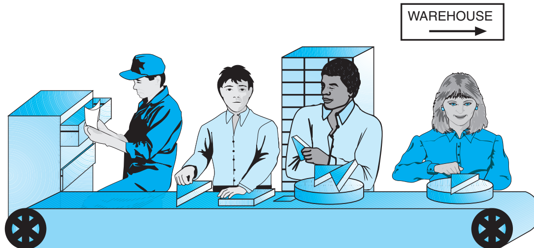
Fig. 8-33 Assembly Line Analogy to Computer Pipeline
